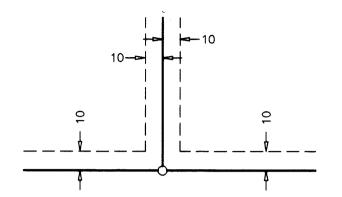
BEING 10 FEET IN WIDTH AND ADJOINING LOT LINES, UNLESS OTHERWISE INDICATED, AND 10 FEET IN WIDTH AND ADJOINING RIGHT OF WAY LINES, UNLESS OTHERWISE INDICATED, AS SHOWN ON THE PLAT
