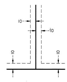
Being 10 feet in width and adjoining lot lines and 10 feet in width and adjoining street lines as shown on this plat upless otherwise shown
