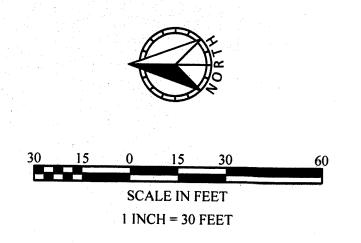
The basis for the bearing system is the north line of Outlot B, LYNWOOD and is assumed to bear South 89 degrees 34 minutes 06 seconds East (See Sheet 2 of 3 Sheets)
