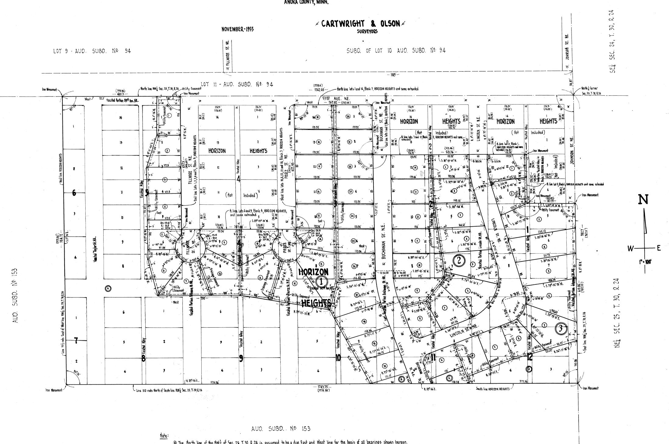
A The North line of the NW\$ of Sec. 25, T.30, R.24 is assumed to be a due East and West line for the basis of all bearings shown hereon.
