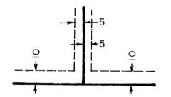
front lot lines, also being 5 feet in width and adjioning side and rear lot lines. inless otherwised noted.
