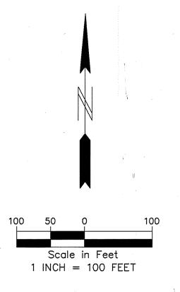
THE ORIENTATION OF THIS BEARING SYSTEM IS BASED ON THE WEST LINE OF THE SW 1/4 OF THE NE 1/4 OF SEC. 24, TWP. 31, RGE. 22, WHICH IS ASSUMED TO HAVE A BEARING OF SOUTH 00°16'47" EAST.
