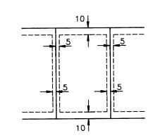
BEING 10 FEET IN WIDTH AND ADJOINING STREET LINES AND REAR LOT LINES, AND 5 FEET IN WIDTH AND ADJOINING SIDE LOT LINES, UNLESS SHOWN OTHERWISE ON THIS PLAT.
