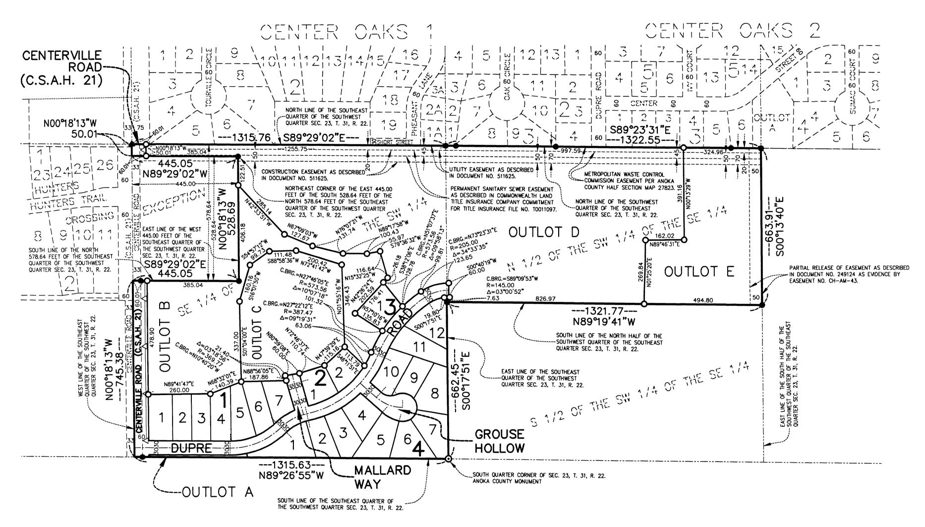
NOTE: ALL MONUMENTS REQUIRED BY MINNESOTA STATUTE AND NOT SHOWN ON THIS PLAT WILL BE SET WITHIN ONE YEAR OF THE RECORDING DATE OF THIS PLAT, AND SHALL BE EVIDENCED BY A 1/2 INCH BY 14 INCH IRON PIPE MARKED BY R.L.S. NO. 12294.
