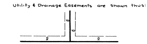
Being lofeet in width and adjoining lot Lines, unless otherwise indicated, and 10 feet in width and adjoining right-of-way and rear Lot Lines, as shown on the plat
