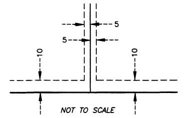
BEING 5 FEET IN WIDTH AND ADJOINING SIDE LOT LINES AND BEING 10 FEET IN WIDTH AND ADJOINING FRONT AND REAR LOT LINES, AND ADJOINING STREETS. EXCEPT AS SHOWN.
