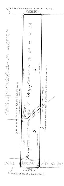
Scale : 1 inch =200 feet. Bearings are on an assumed datum. o Denotes iron pipe set with a plastic plug stamped RLS 13057.
