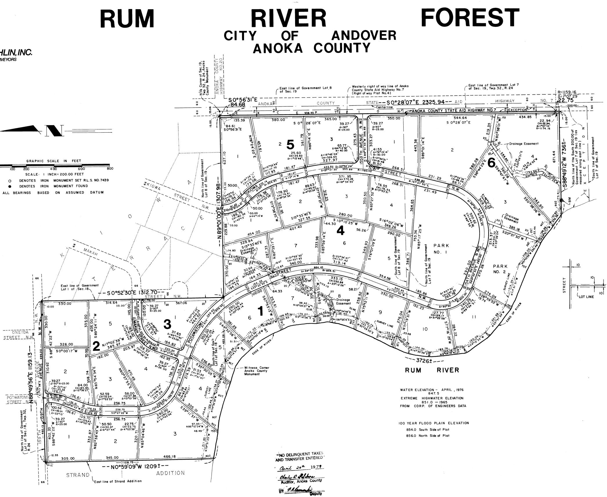
BM. ELEVATION = 849.40 SEA LEVEL DATUM Railroad spike in east face of twin 14," Maples on south line lot 4 block 6,60±feet east of survey line.
