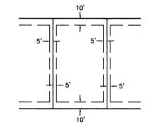
BEING 10 FEET IN WIDTH AND ADJOINING STREET LINES AND REAR LOT LINES, AND 5 FEET IN WIDTH AND ADJOINING SIDE LOT LINES, UNLESS SHOWN OTHERWISE ON THIS PLAT.
