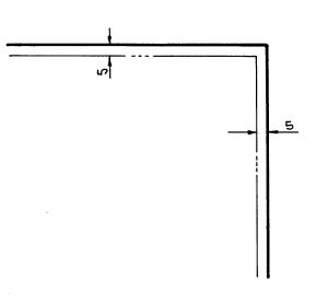
UTILITY AND DRAINAGE EASEMENT SHOWN THUS BEING 5.0 FEET IN WIDTH AND ADJOINING LOT LINES AS SHOWN ON THIS PLAT.
