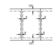
BEING 10 FEET IN WIDTH AND ADJOINING STREET LINES AND REAR LOT LINES, AND 5 FEET IN WIDTH AND ADJOINING SIDE LOT LINES, UNLESS SHOWN OTHERWISE.
