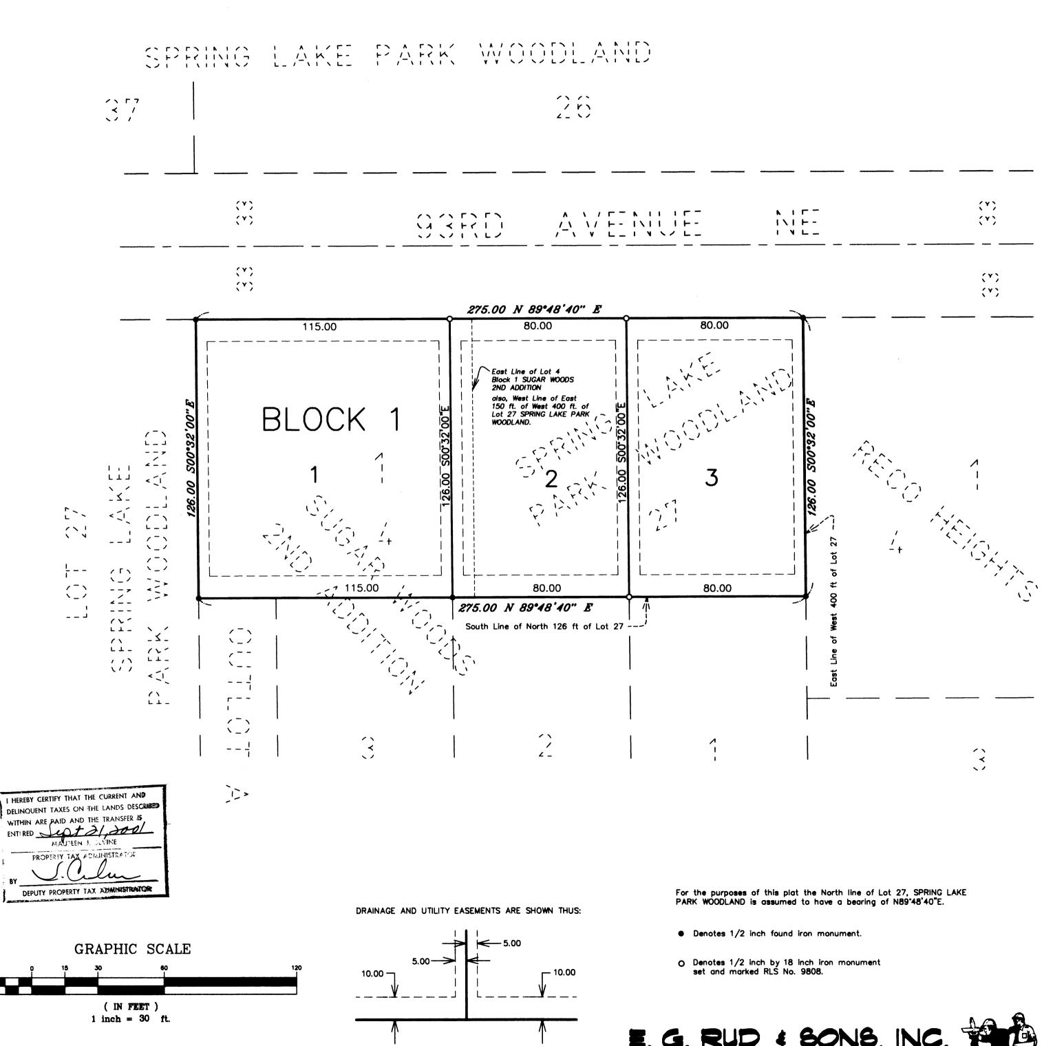
BEING 5 FEET IN WIDTH AND ADJOINING SIDE LOT LINES AND BEING 10 FEET IN WIDTH AND ADJOINING STREET AND REAR LOT LINES UNLESS OTHERWISE SHOWN ON THIS PLAT.
