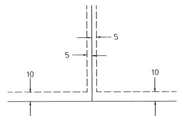
being 5 feet in width, unless otherwise indicated, and adjoining lot lines, and 10 feet in width and adjoining street lines, as shown on the plat.
