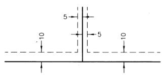
being 5 feet in width, and adjoining lot lines, and 10 feet in width and adjoining right of way and rear lot lines unless otherwise shown on the plat.
