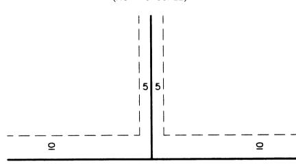
BEING 10.00 FEET IN WIDTH AND ADJOINING RIGHT-OF-WAY LINES, BEING 5.00 FEET IN WIDTH AND ADJOINING LOT LINES, AND BEING 15.00 FEET IN WIDTH AND ADJOINING REAR LOT LINES UNLESS OTHERWISE SHOWN ON THE PLAT.
