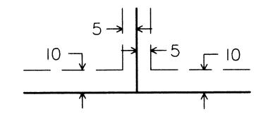
BEING 5.00 FEET IN WIDTH, AND ADJOINING LOT LINES, AND BEING 10.00 FEET IN WIDTH, AND ADJOINING RIGHT-OF-WAY LINES AND REAR LOT LINES UNLESS OTHERWISE SHOWN ON THE PLAT.
