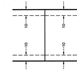
DRAINAGE AND UTILITY EASEMENTS BEING 10 FEET IN WIDTH, UNLESS OTHERWISE INDICATED, ADJOINING FRONT AND REAR LOT LINES, AS SHOWN ON THIS PLAT.
