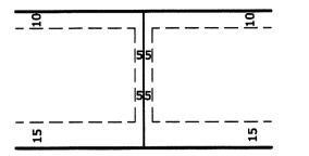
BEING 15 FEET IN WIDTH ADJOINING ALL RIGHT OF WAY LINES, AND BEING 5 FEET IN WIDTH ADJOINING ALL SIDE LOT LINES AND BEING 10 FEET IN WIDTH ADJOINING ALL REAR LOT LINES, UNLESS OTHERWISE SHOWN ON THIS
