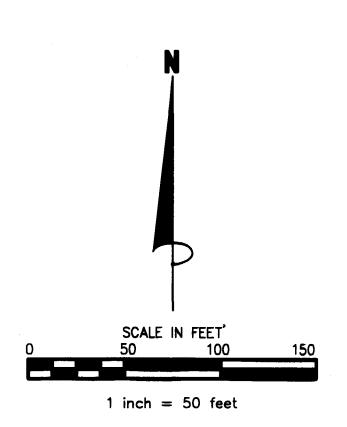
BEARINGS ARE BASED ON THE NORTH LINE OF SOUTHEAST QUARTER OF THE SOUTHEAST QUARTER OF SEC. 16, T. 32, R. 25, WHICH IS ASSUMED TO HAVE A BEARING OF S 89°24'10" E.
