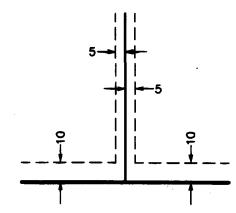
DRAINAGE AND UTILITY EASEMENTS BEING 5 FEET IN WIDTH, UNLESS OTHERWISE INDICATED, ADJOINING LOT LINES, AND BEING 10 FEET IN WIDTH, UNLESS OTHERWISE INDICATED, ADJOINING RIGHT OF WAY LINES, AS SHOWN ON THE PLAT.
