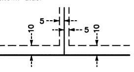
Being 5 feet in width and adjoining lot lines, unless otherwise shown, and 10 feet in width and adjoining street lines as shown on the plat.
