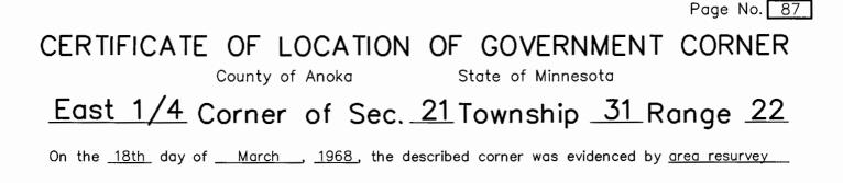
and to perpetuate the location of said corner, at the exact location thereof, a permanent marker was placed consisting of <u>a cast iron monument 30'± West of Lake edge</u>
