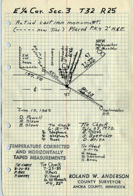
straight line and on prorated distance from old Survey dist. between N. E. Cor & S. E. Cor Sec 3. S. W. Cox Box-elder N&W. House PKin metal calver Telephone
