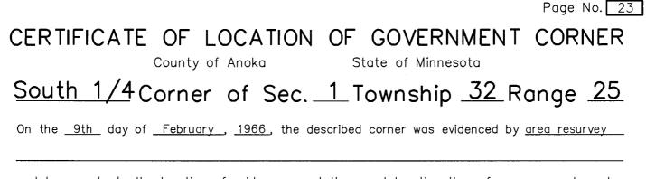
and to perpetuate the location of said corner, at the exact location thereof, a permanent marker was placed consisting of <u>a cast iron monument with a sign and post on the south side</u>
