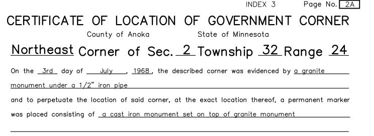
AND on the <u>17th</u> day of <u>July</u>, <u>2023</u>, said permanent marker was <u>reset with 8" CIM set in</u> <u>concrete after road construction. Verified position by ACS RTK GPS mehod & updated ties after setting</u>.
