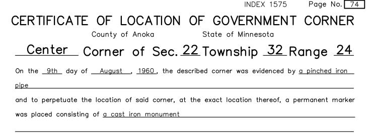
AND on the <u>23rd</u> day of <u>June</u>, <u>2022</u>, said permanent marker was <u>found broken off and</u> <u>replaced with new cast iron monument flush. Verified position by VRS GPS methods. Updated ties.</u> Updated reference ties are as shown below.
