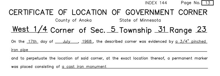
AND on the <u>19th</u> day of <u>May</u>, <u>2022</u>, said permanent marker was <u>found paved over and</u> <u>broken down 0.8'±</u>. Removed old CIM and reset with new CIM set flush to surface. Updated ties. Updated reference ties are as shown below.
