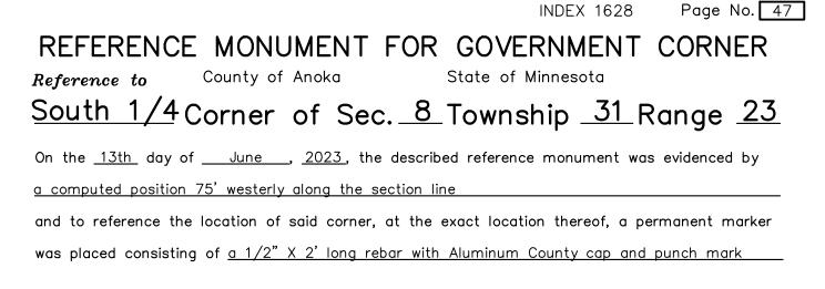
AND on the <u>13th</u> day of <u>June</u>, <u>2023</u>, said permanent marker was <u>set up 0.2'± using RTK</u> <u>GPS method and ties were established to the reference monument</u>
