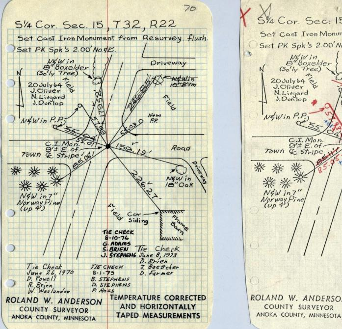
30 54 Cor. Sec. 15 , T32, R22 Set Cast Iron Monument from Resurvey. flush Set PK Spk's 2.00' No. &E. Driveway Road Cor Siding R. Brien W. Westander TEMPERATURE CORRECTED ROLAND W. ANDERSON AND HORIZONTALLY TAPED MEASUREMENTS
