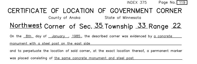
AND on the <u>6TH</u> day of <u>July</u>, <u>2023</u>, said permanent marker was <u>removed concrete mon</u>ument <u>& replaced with 2" sq Telspar w/ aluminum cap can punch mark, set up 1.5'±. No Ties available</u>.
