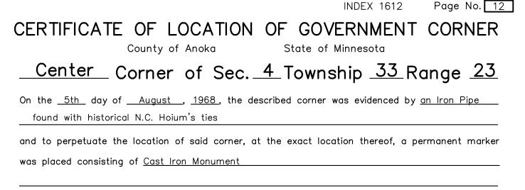
AND on the <u>29th</u> day of <u>June</u>, <u>2023</u>, said permanent marker was <u>found down 1.7'. Postion</u> verified by ACS RTK GPS. Added partial CIM on top of existing position, set flush. Ties established. Updated reference ties are as shown below.
