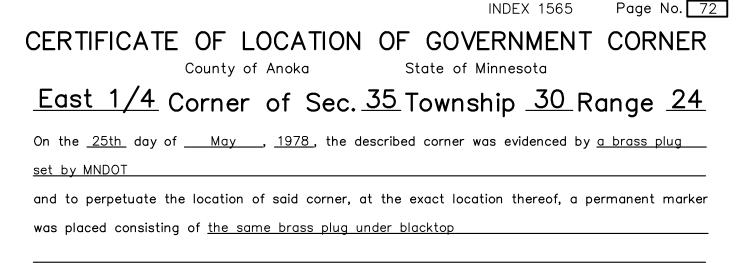
AND on the <u>27th</u> day of <u>October</u>, <u>2022</u>, said permanent marker was <u>not found</u>. Set a <u>1/2</u>" iron pipe w/cap flush using area resurvey. Verified position by VRS GPS methods. Updated ties.
