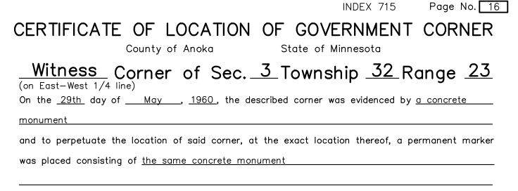
AND on the <u>6th</u> day of <u>February</u>, <u>2023</u>, said permanent marker was <u>found up 0.5'± with a</u> <u>P.K. nail in top of monument. Position Coordinates were verified using County RTK GPS method.</u>
