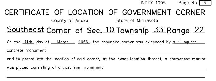
AND on the <u>10th</u> day of <u>March</u>, <u>2023</u>, said permanent marker was <u>found up 0.2'± and</u> the position was verified as correct using County RTK GPS method
