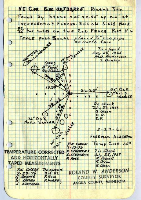
NE COR SEE 33,733,825 BURNS TUN Found Sq. Stone 0.35 x 0.45 up 0.2' A+ intersect of Fences. SEE old field Book BT FOR notes on this COR. FENCE POST No FENCE POST South placed 1/2" iron Pipe on N.fac 30" OAK 36.23 Naila WAShER 3-29-61 FREEMAN ANDERSON TEMP CORR 350 AND HORIZONTALLY TAPED MEASUREMENTS COUNTY SURVEYOR Tie check AMOKA COUNTY, MINNESOTA J. Dunlop
