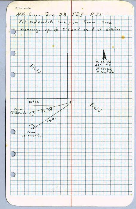
N1/4 Gr. Sec. 28-T33-R25 The Right of Won. with warning sign 20.10 N M.D. Anderson H.J. Layson temp. 750 tape 10 TEMPERATURE CORRECTED COUNTY SURVEYOR
