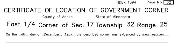
and to perpetuate the location of said corner, at the exact location thereof, a permanent marker was placed consisting of <u>a cast iron monument</u>
