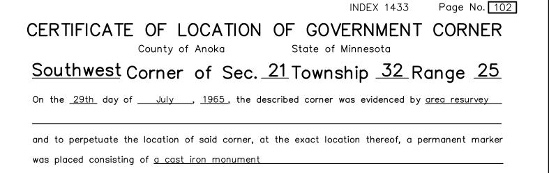
AND on the <u>12th</u> day of <u>May</u>, <u>2023</u>, said permanent marker was <u>set cast iron</u> monument after road construction, verified position using RTK GPS methods. Updated ties.
